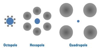
Figure 2. Relative size, internal diameter and ion stability regions (in blue) for multipole ion guides (octopole, hexapole and quadrupole)
