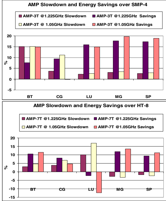
Figure 2: AMP slowdown and energy savings for NAS benchmarks over SMP-4 and HT-8 at 1.4GHz.
