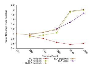
Figure 10: Fire Dynamics Simulator Scaling Results for Nehalem
