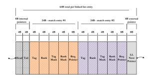
Figure 2: Packing data structures into 64 byte cache lines
