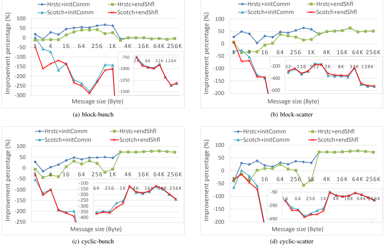
Fig. 3. Micro-benchmark performance improvements for non-hierarchical topology-aware allgather with four different initial mappings and 4096 processes.
