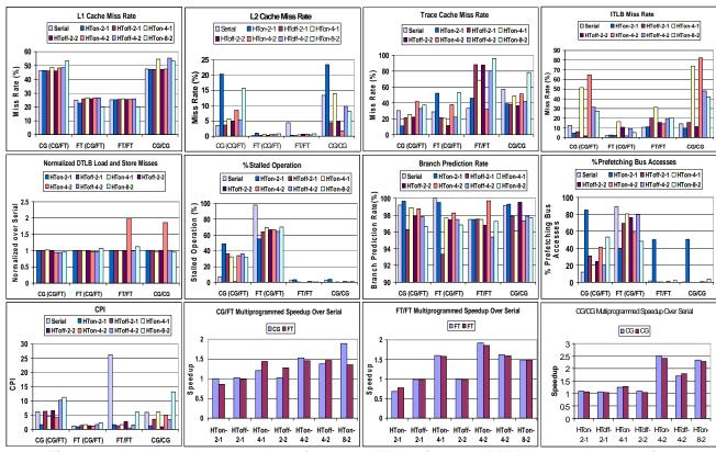
Figure 4. L1, L2, and trace cache miss rates, ITLB miss rate, DTLB load and store misses normalized to serial case, % of execution spent in a stalled state, branch prediction rate, % of prefetching bus accesses, and CPI and speedup of multi-program workloads.
