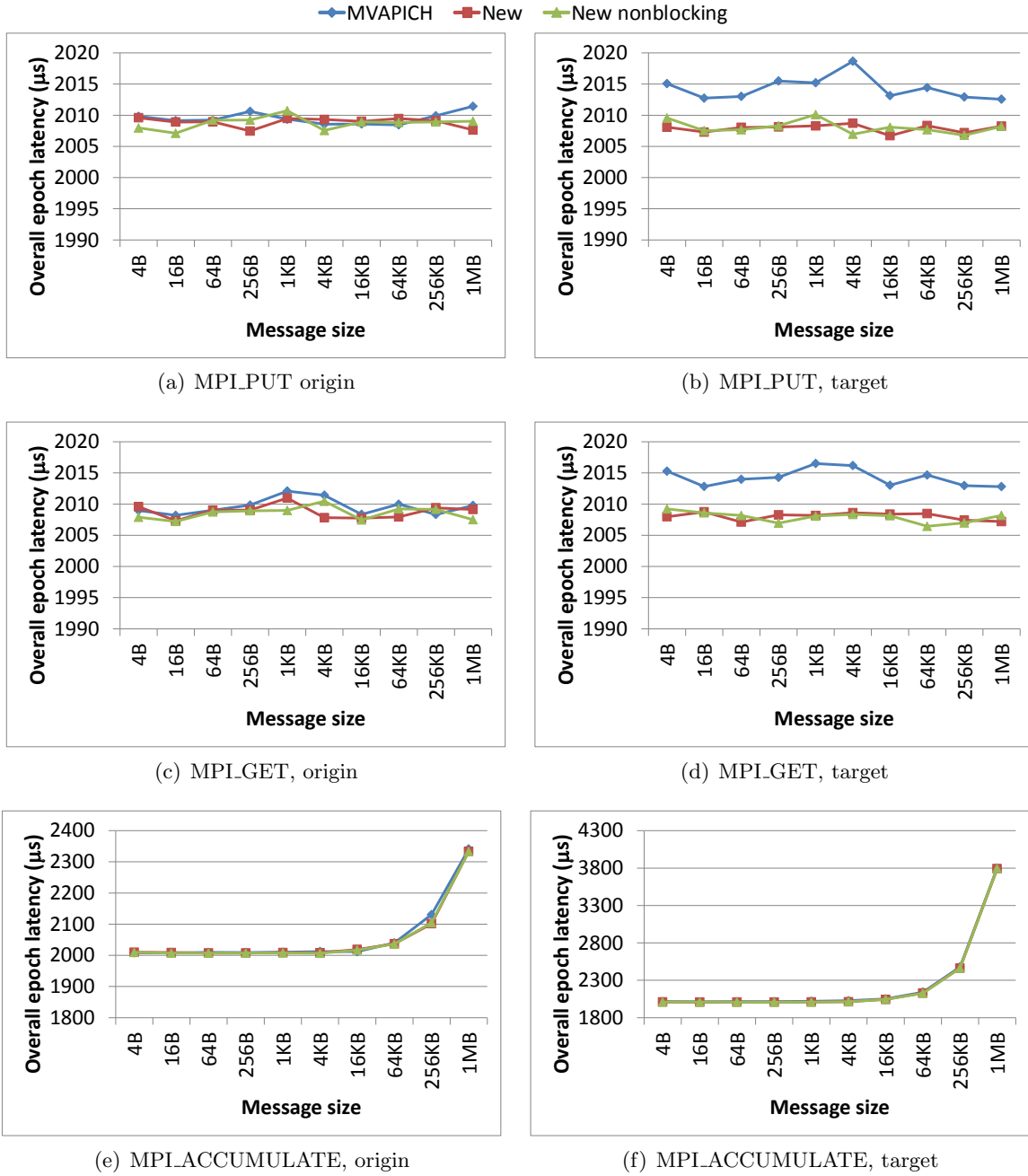
Figure 5.11: Fence comparative communication/computation overlapping of MVAPICH, blocking and nonblocking versions of the new design
