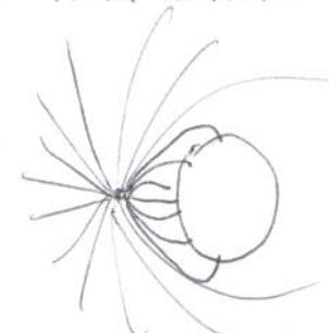
point charge near conducting sphere at fixed potential  $V$
