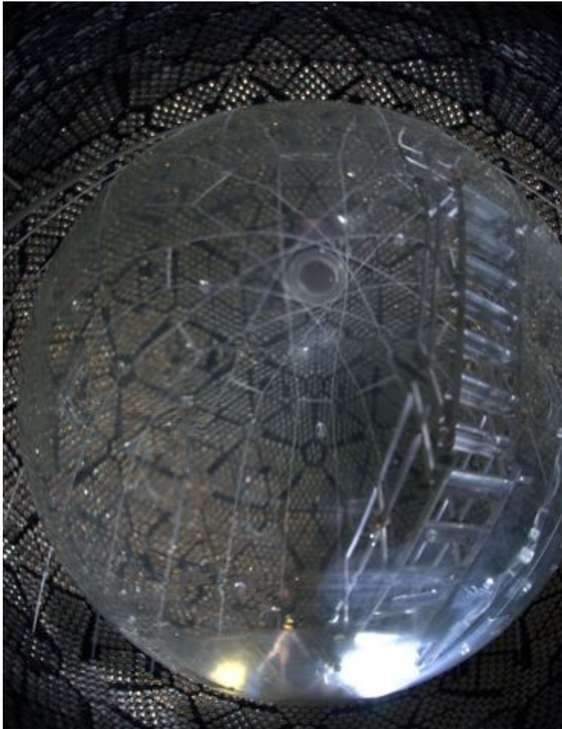
Rotating ladder for lower hemisphere
