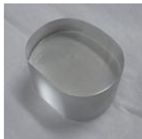
^{40}\text{Ca}^{100}\text{MoO}_4 crystal ^{100}\text{Mo} is a source of 0\nu\beta\beta
