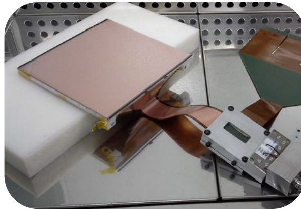
First batch of 20 cm square MicroMegas modules made and commissioned
