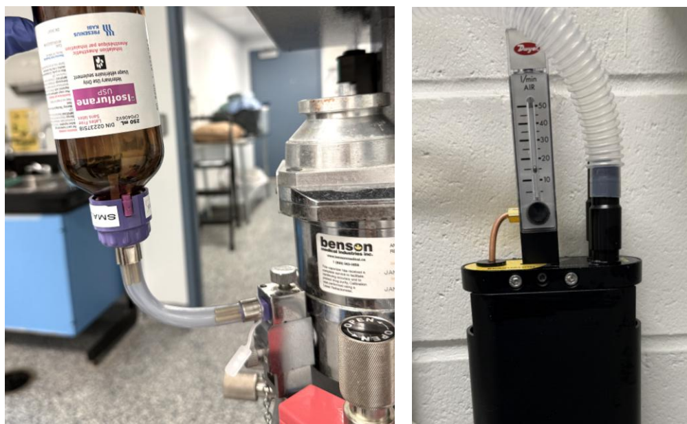
Image of isoflurane key filler bottle adaptor (left) and Moduflex set to 15 LPM (right)
