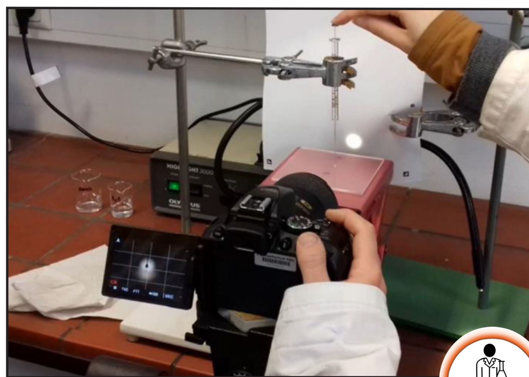
Figure 2: Example of a simple practical exercise to collect images of the contact angle of surfactant solutions with different concentrations (photo credits Lisbach, Ocello, Nemeth, Wiefel)
