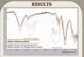
FTIR spectroscopy – Unexpected results as bands in 3330 and 1025 regions show increase in -OH and C-OH stretching, indicating oxidation, in all samples *except* the O<sub>3</sub> exposure from Munters, which shows a decrease but no carbonyl groups. Oxidation from H<sub>2</sub>O<sub>2</sub> and Ca(ClO)<sub>4</sub> appears in reverse of what was expected. Queen's O<sub>3</sub> samples show marked increase in -OH and also a small shoulder indicating carbonyl groups.
