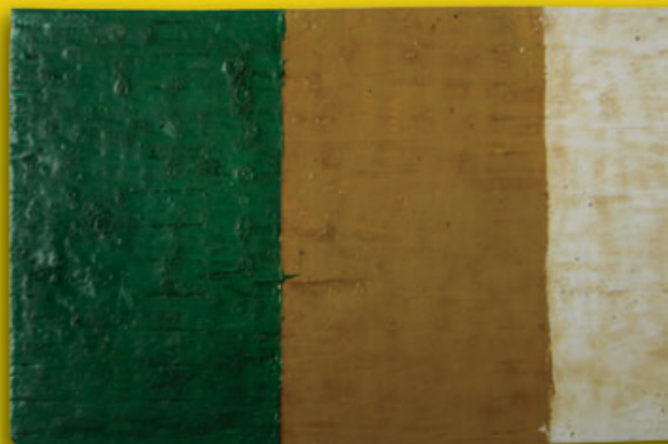
Above: Samples of glass, brick and wood, varnished with Genesis Coatings Graffiti Melt, after heat aging, light aging, and humidity fluctuations for a period of 49 days.
