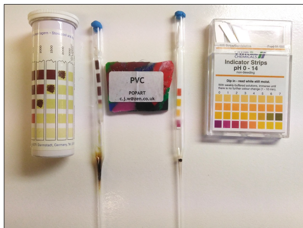
Micro-Oddy tests within sealed glass pipettes for rapid testing of packing, storage and display materials
