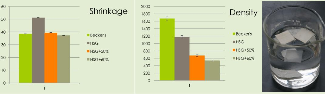
Fig. 1) The Becker's Latex Spackle sample sink s in water, because of its comparatively higher density; the other three samples flo
