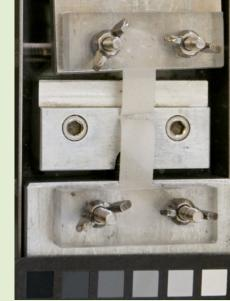
Fig. 2) Torn HSG + 50% PVC sample during tensile testing
