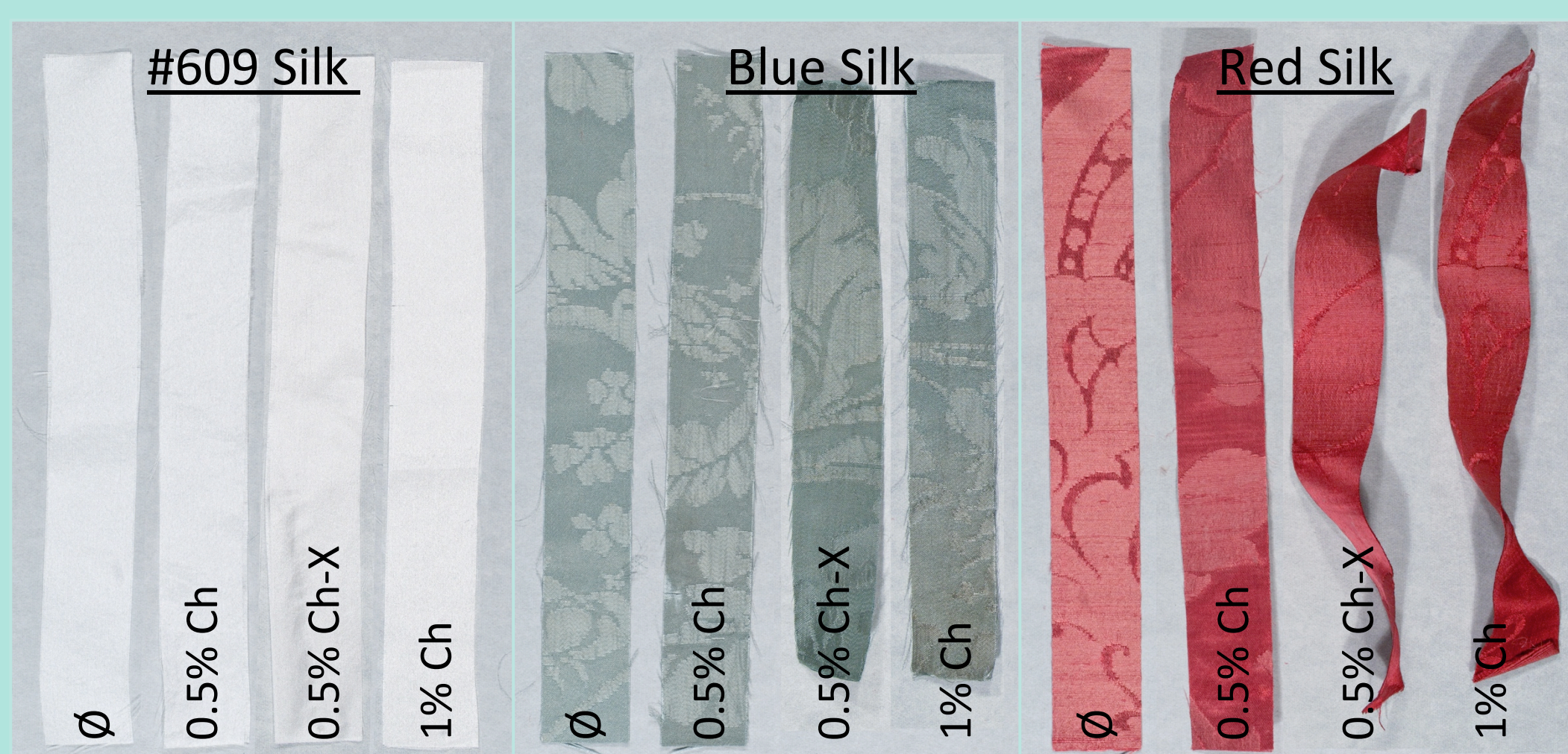
Comparisons of experiment conditions. Treated silks darkened, and some curled and twisted.
