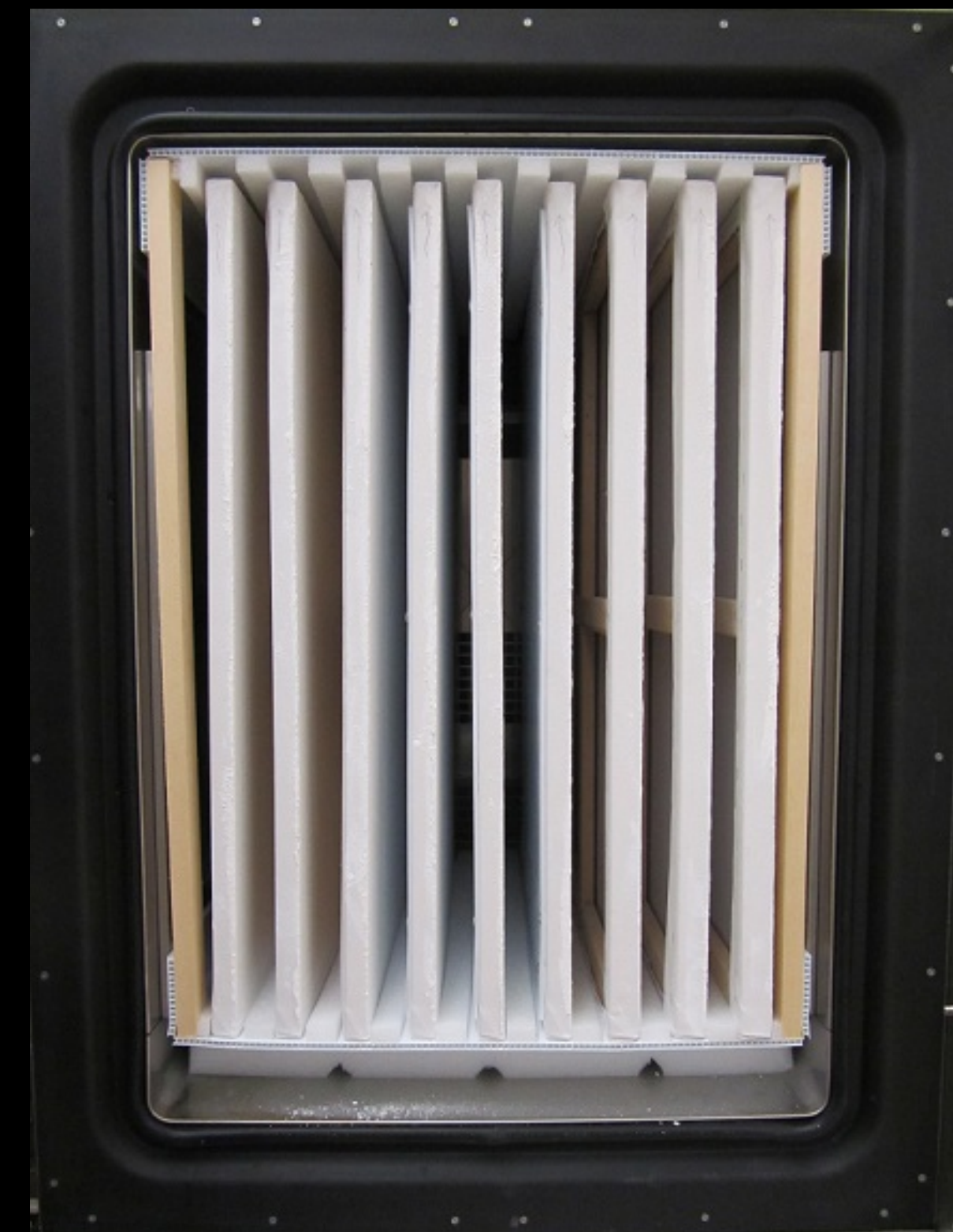
Fig. 1 Samples in the Espec ESL-3CA environmental chamber
