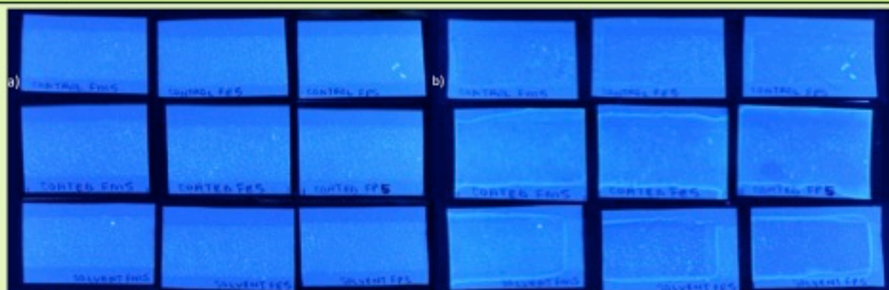
Figure 2: Samples exposed to Ultraviolet light a) before gellan gum application b) after two applications of gellan gum
