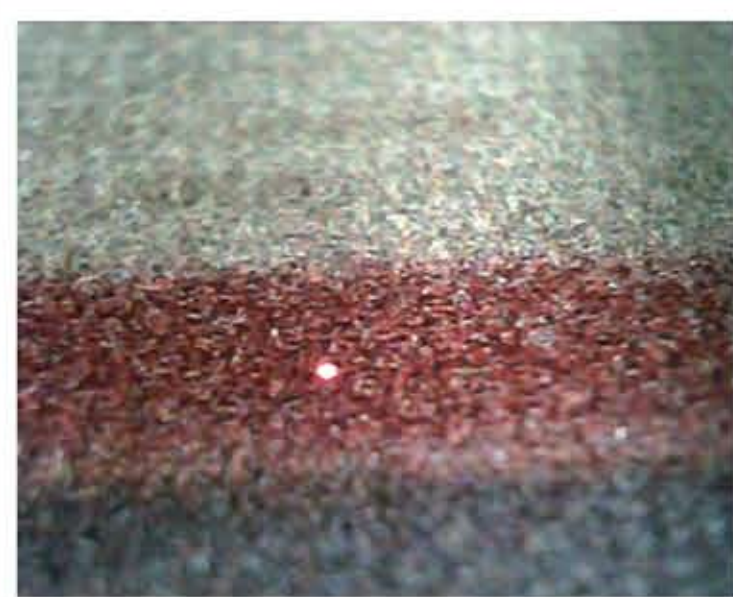
Fig 4: Red being tested. The beam of light must hit a target thread at its highest point in the weave in order to have maximum reflectance.
