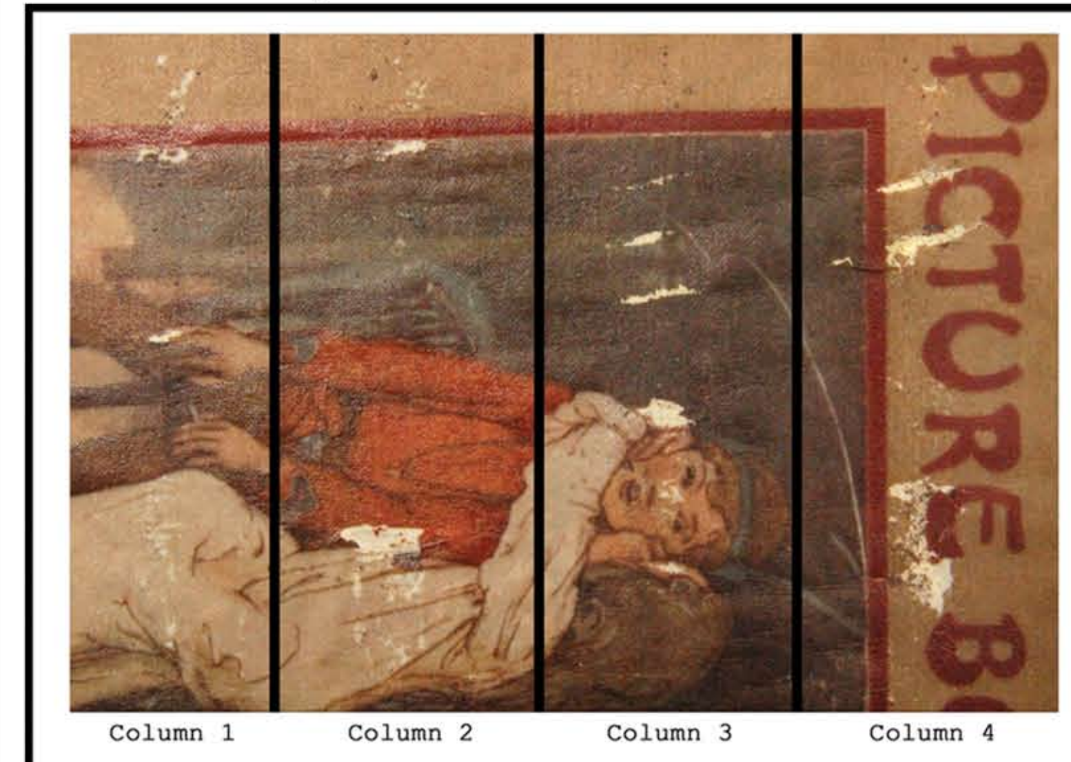
Fig 6: To test the wetfastness of the UV curable inks, a sample was first left to soak in water for 24 hours. Four columns were drawn and a piece of blotter paper held at even pressure was rubbed across the surface of each column. Column 1 was rubbed two times, column 2 was rubbed four times, and so on. There was very heavy ink losses present in all columns. The same rubbing setup was used to test for dryfastness with insignificant ink transfer.
