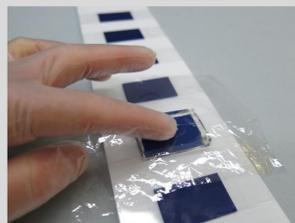
Fig.3 Testing of gellan gum cleaning system on a coupon
