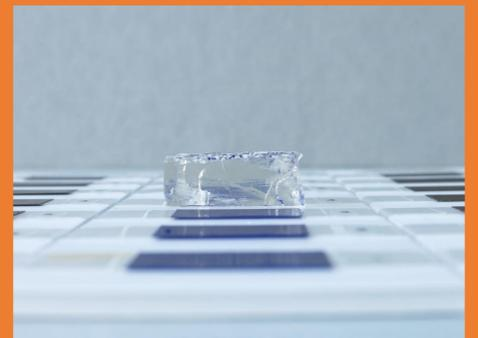
Fig.7 Rigid KELCOGEL® CG-LA hydrogel gellan gum cleaning system containing ECOSURE™ EH-9 surfactant, application of the gel cut to size on a W&N Finity ultramarine blue acrylic paint coupon
