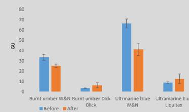
Fig.10 Gloss before and after testing with ECOSURF EH-9 gellan gum cleaning system
