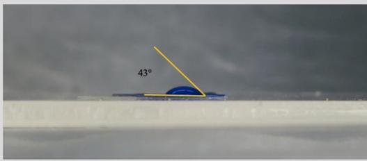
Fig.2 Contact angle testing was performed for each paint sample types
