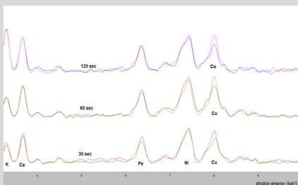
Fig.5 XRF spectra showing that copper metal is extracted after contact between gellan gum containing EDTA and a copper foil
