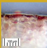
Fig.3 Mixture of oxblood, casein and lime over pine wood
