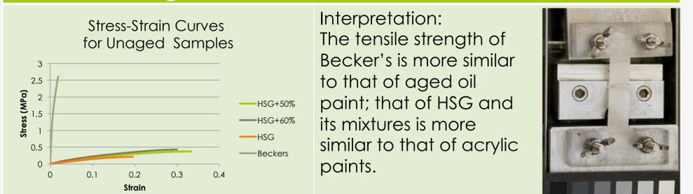
Fig. 2) Torn HSG + 50% PVC sample during tensile testing
