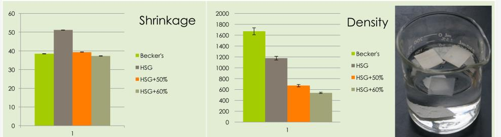
Fig. 1) The Becker's Latex Spackle sample sink s in water, because of its comparatively higher density; the other three samples float.
