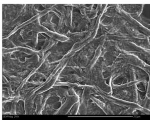
Fig. 11. SEM (Mag. 250x) of Mg aggregate on Stonehenge paper treated with 2.25% w/v Laponite with 0.25% w/v xanthan gum with rayon barrier tissue.
