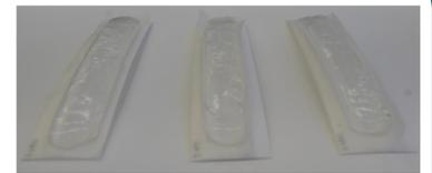
Fig. 1. Paper samples being treated with Laponite poultice through barrier tissue.
