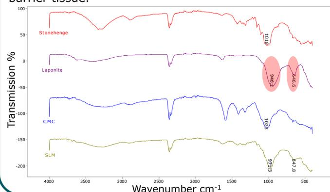
Fig. 12. (From top to bottom) FT-IR spectra: Stonehenge paper; Laponite with characteristic peaks highlighted; CMC; Stonehenge paper treated with 2.25% w/v Laponite with 0.25% CMC through lens tissue carrier.
