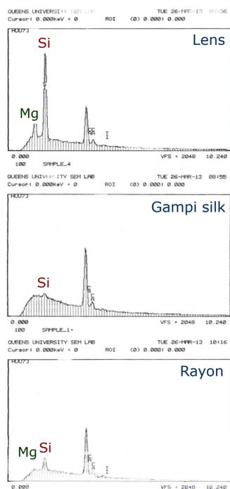
Figs. 7, 8, 9. (From top to bottom) EDS spectra of Stonehenge paper samples treated with 2.25% w/v Laponite with 0.25% w/v CMC.
