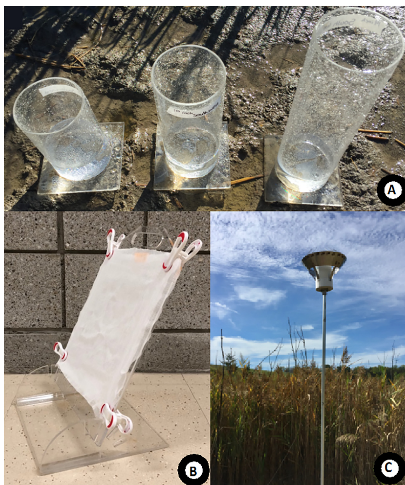
Fig. 1. A) Collection columns, 17.8, 25.4, and 35.6 cm in height. B) Cheesecloth mount ( 24 \times 24 \text{ cm} ) with all-plastic clothespins. C) Environment Canada dustfall sampler.
