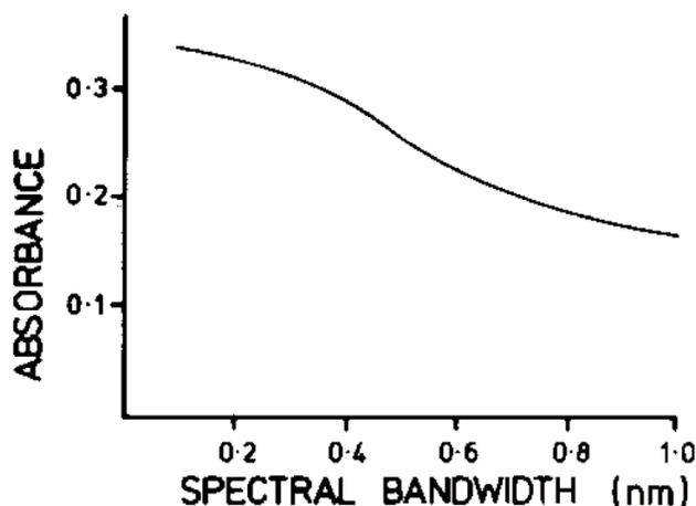
Figure 9. Sensitivity as a function of spectral bandwidth for Sb at 217.6 nm.
