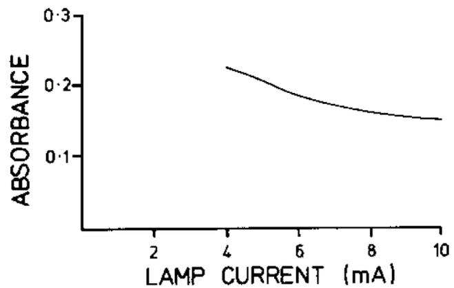
Figure 4. Sensitivity as a function of current for Cd at 228.8 nm.
