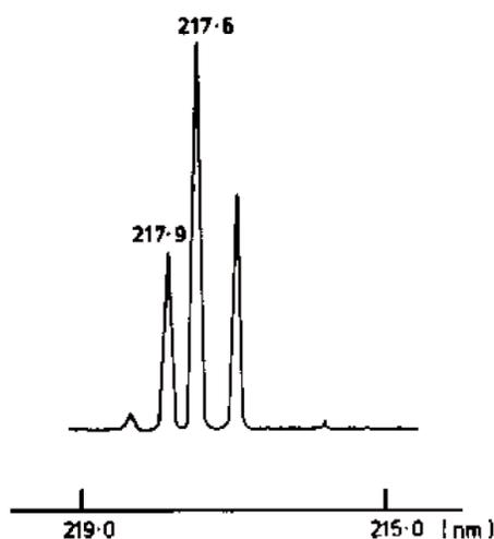
Figure 8. Spectral scan of Sb lamp in the vicinity of the 217.6 nm resonance line.
