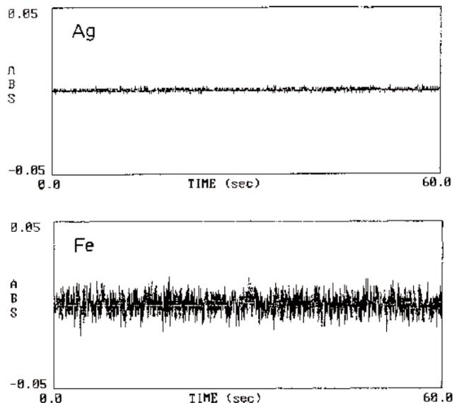
Figure 7. Inherent noise levels of Ag and Fe hollow cathode lamps operated under recommended conditions.
