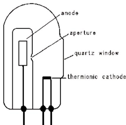
Figure 10. Deuterium lamp construction.
