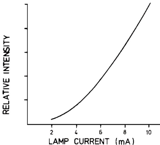
Figure 2. Intensity as a function of lamp current for Cd at 228.8 nm.
