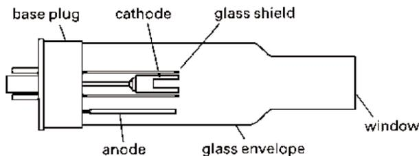
Figure 1. Hollow cathode lamp construction.
