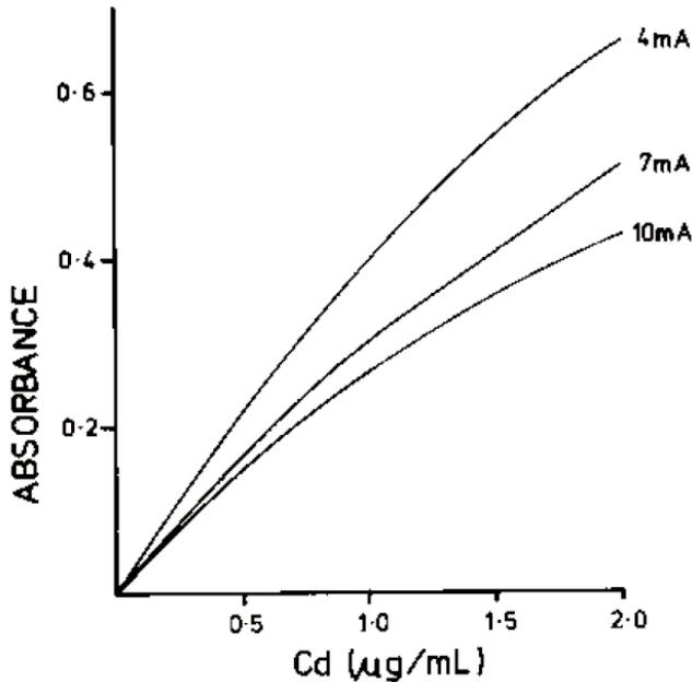
Figure 5. Calibration graphs for a Cd hollow cathode lamp operated at various currents.
