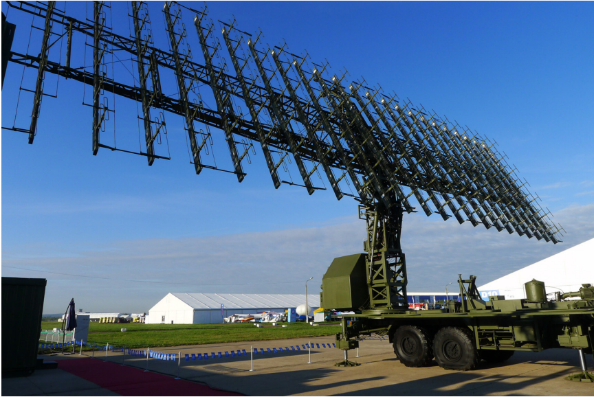
This Nizhny-Novogorod Research Institute (NNIIRT) 55Zh6ME radar system was on display at the August 2013 MAKS airshow at Zhukovsky, just outside of Moscow. It features VHF, L-band and S-band modules that are all part of an integrated radar system. Each module contains an active, electronically scanned array (AESA) radar. (AW&ST / Bill Sweetman Photo)
