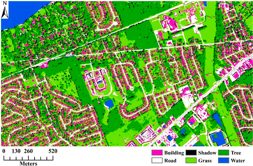
Figure A12. Classification map generated by combining classification maps of the MLP model for the 30 cm image.
