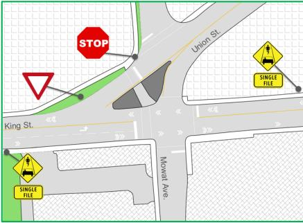
**Figure 10.13:** An illustration of the recommended improvements to the intersection of King Street with Union Street and Mowat Avenue.
