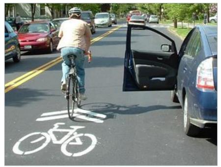
**Figure 7.6:** Example of a sharrow showing rider location within the roadway that safely avoids the opening car door (CAN, 2012).
