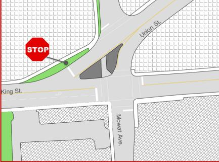
Figure 10.12: An illustration of the current condition of the intersection of King Street with Mowat Avenue and Union Street. Sidewalks are shown in white, and the pedestrian island in the middle of the intersection is shown in dark grey. A popular fast food restaurant is located near the southwest corner of the intersection.
