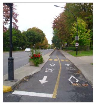
Image 76: Example of a bidirectional bike lane separated from the road by a median (Riddell, 2013).
