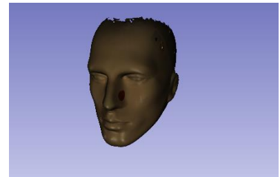
Figure 1: 3D Surface scan of mannequin head, with sticker on nose representing a skin lesion.
