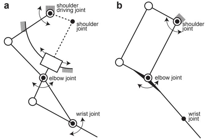
Fig. 2. Top view schematics of (a) Planar MEDARM and (b) KINARM. KINARM is supported only at the shoulder joint, while Planar MEDARM is supported and guided by its curved track, creating a virtual 4-bar linkage (see dashed lines in (a)). The other major difference is that Planar MEDARM offers a third DOF at the wrist, while KINARM does not.
