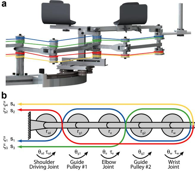
Fig. 3. (a) A CAD drawing showing the cable routing scheme used for the Planar MEDARM. (b) A simplified planar schematic representation of the optimal cable routing structure. Each of the four cables is denoted by a different colour. Symbols  $s$ ,  $\xi$ ,  $r$ ,  $\tau$  and  $\theta$  represent cable displacement, cable force, pulley radius, joint torque and joint angle respectively.
