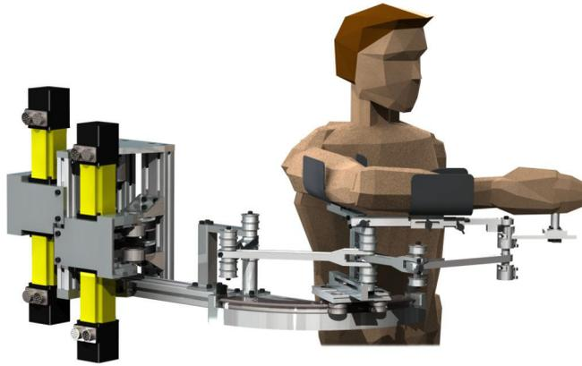
Fig. 1. A CAD drawing of the Planar MEDARM. The 3DOF mechanism is entirely underneath the user's arm. The cable-drive system allows the motors to be located behind the user (cables not shown).
