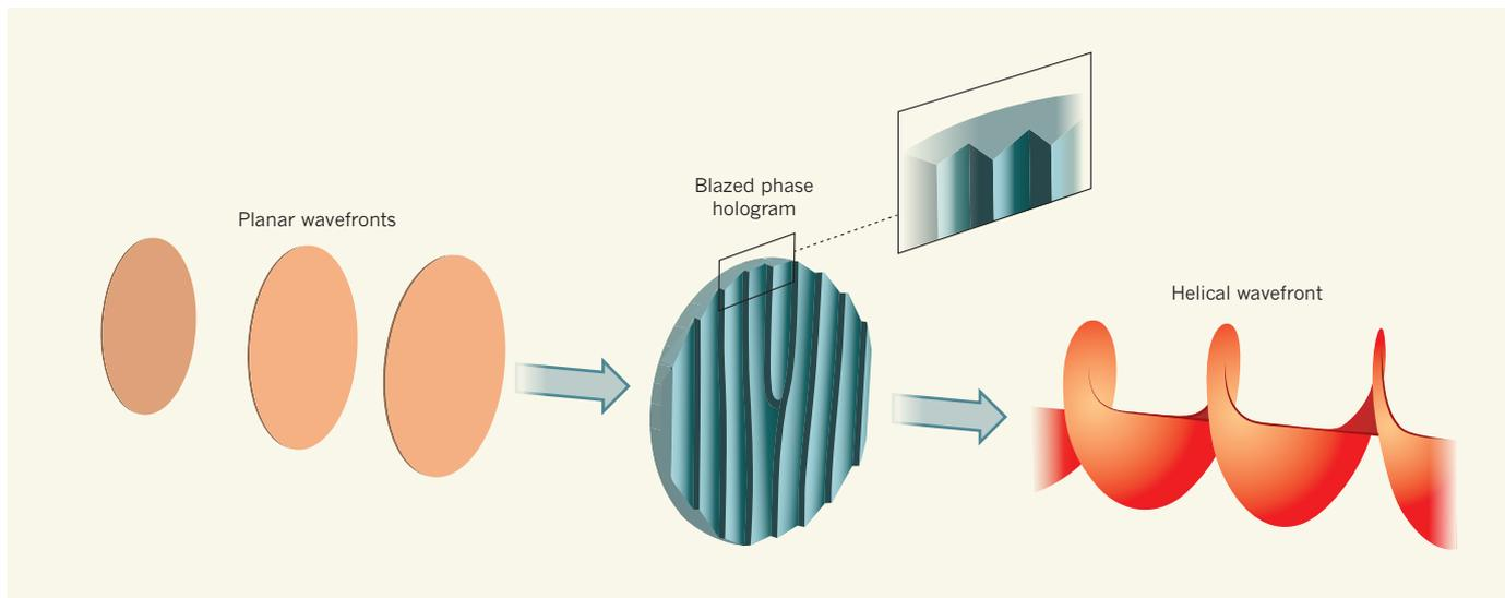
**Figure 1 | Converting wavefronts.** Grillo *et al.*<sup>6</sup> have designed a blazed phase hologram that has a sawtooth-thickness structure. The device converts an electron beam in which the wavefronts form planes into a beam with a wave crest that rotates about its axis of propagation, tracing out a helical wavefront.
