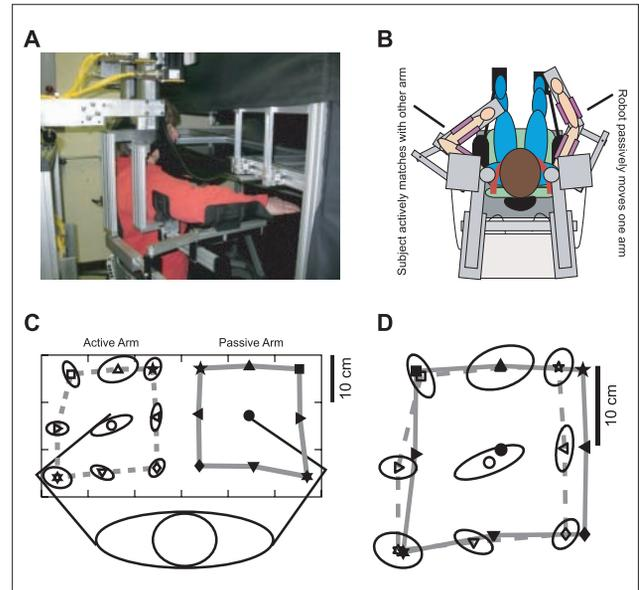
**Figure 1.** KINARM robotic device. (A and B) Picture and schematic of device. (C) Typical control subject data. The right hand was actively moved to 9 spatial locations by the robot (filled symbols). The subject mirror matched with the left hand (open symbols). Ellipses around the targets represent 1 standard deviation. (D) Data from right hand are mirror transformed to quantify discrepancies between the passive robotically moved hand position and the active hand position.
