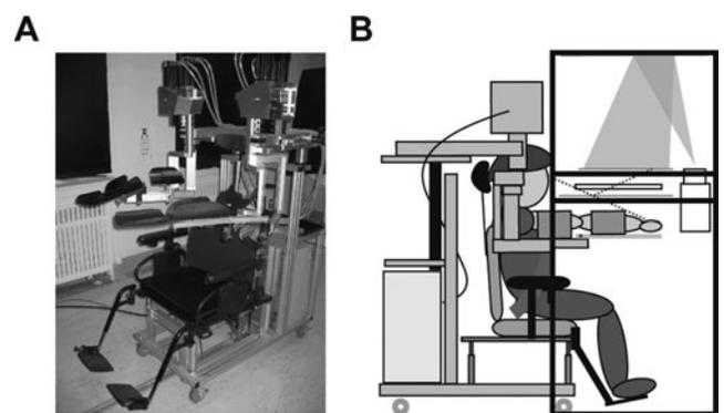
**Figure 1.** Apparatus. A, Photograph of the KINARM exoskeleton robot, showing the modified wheelchair base and exoskeletal arm troughs linked to motors mounted up top. B, Schematic diagram illustrating the KINARM exoskeleton robot docked to the augmented reality workstation in which subjects view targets projected through a semitransparent mirror onto the same plane as their arms and hands.
