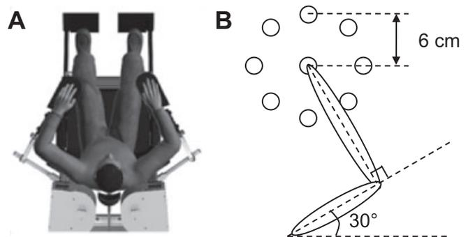
**Fig. 1.** KINARM robotic device. **(A)** Picture and schematic of device, showing a top-down view with a virtual subject sitting in the chair and resting their arms in the robotic exoskeleton. **(B)** Children moved from the central target, set at 30° of shoulder extension and 90° of elbow flexion, to 8 surrounding targets in a 6 cm radius.
