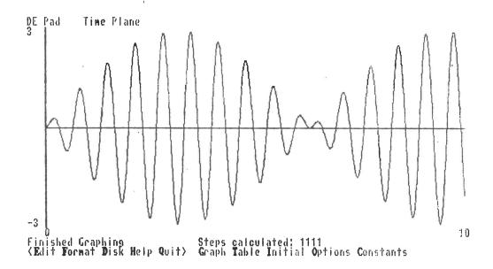
The program allows the user to choose which variables are to be plotted and over what range. The program also provides a variety of supplementary facilities: for instance, functions, constants and comments may be entered; constants and initial conditions can be directly changed to study corresponding changes in a solution; and values of the solution may be displayed in a table.
