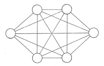
ach other, a result from COMBINATORICS says that the number of pieces of wire would have to be n(n-1)/2, where n is the number of telephones. There are about 15,000,000 telephones in Canada alone in 1979; this means that about 112,000,000,000,000 pieces of wire would be needed if the original connection process had been continued.
