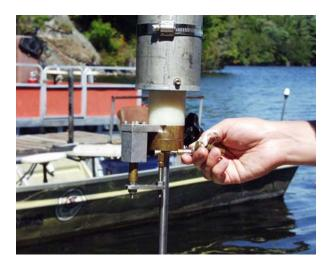
Use extruder key (1.0cm) to adjust extruder to desired extruding interval. Adjust set screw to automatically drop extruder to prescribed interval.
