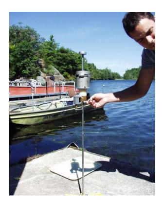
Set up extruder on level surface. Make sure that the rod is straight.
