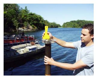
Push sediment up one interval at a time, and scrape sediment slice into labelled bag. The first few slices will be extremely watery.
