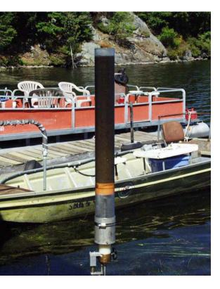
If quick removal of water is necessary while siphoning, push the core tube firmly but slowly against the extruding rod. This will raise the sediment toward the top of the core tube.
