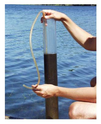
Use the siphon tube to begin to remove water above the sediment. Ensure bottom of siphon does not disturb top layer of sediment.
