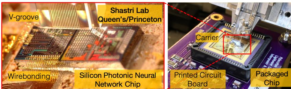
Our fabricated silicon photonic neuromorphic chip packaged with optical and electrical I/O and mounted on a printed circuit board which can be interfaced with a microcontroller to program the chip with machine learning libraries (e.g. TensorFlow and PyTorch).
