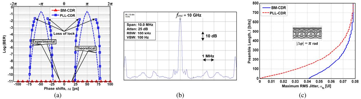
Fig. 2. (a) BER performance of the BM-CDR (compared to a conventional PLL-based CDR) versus phase step for zero preamble length. (b) Recovered clock spectrum. (c). Preamble length versus rms jitter to achieve BER  $< 10^{-10}$ .
