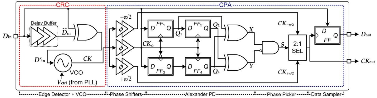
Fig. 1. Block diagram of the proposed BM-CDR.
