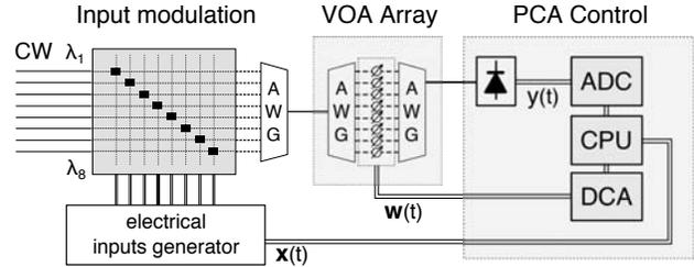
(a) Demonstrated batch PCA experiment via software-driven Oja’s rule.
