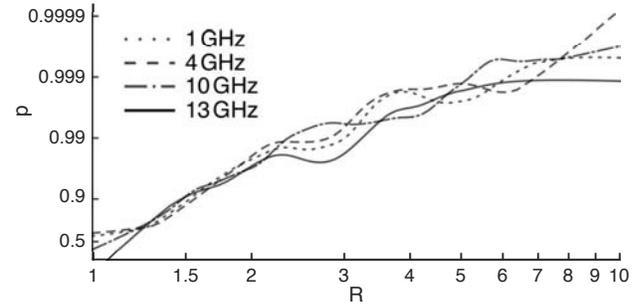
(b) Performance results as a function of different input bandwidth and eigenvalue ratios.
