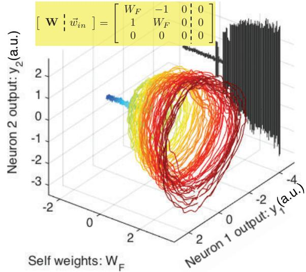
Fig. 3. A supercritical Hopf bifurcation involving two nodes and no input. Off-diagonal weights are asymmetric, and diagonal self weights are swept in concert. A transition between stable and autonomous oscillation is observed. Color represents self weight value.
