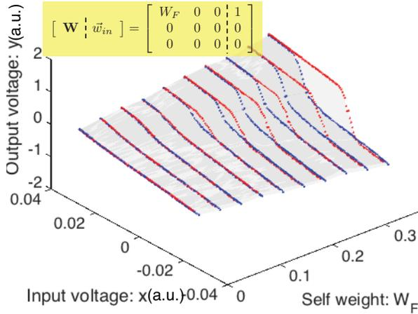
Fig. 2. A cusp bifurcation with a single node with self-connection and an external input. A sweep of self-weight strength,  $W_F$ , is controlled by a MRR weight. Blue points: increasing input voltage. Red points: decreasing input voltage. The transition from stable to bistable is parameterized by the weight.
