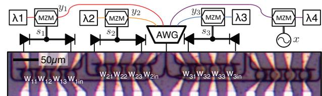
Fig. 1. Experimental setup with three MZM neurons, wavelength-multiplexed in an AWG and coupled into an on-chip broadcast-and-weight neural network.  $\lambda_4$  carries an external input derived from a signal generator. The 3x3 recurrent network state is configured by MRR weight banks.
