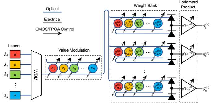
Fig. 1. Photonic architecture implementing the DFA training algorithm. The gradient of the hidden layer  $k$  is calculated through the matrix-vector product of the  $M \times N$  matrix  $\mathbf{B}^{(k)}$  and the output layer gradient vector  $\mathbf{e}$  of size  $N$ . The Hadamard product  $\mathbf{B}^{(k)} \mathbf{e} \odot g'(\mathbf{a}^{(k)})$  is executed using TIAs, yielding the desired vector  $\delta^{(k)}$  in the electrical domain.
