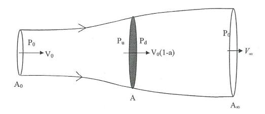
Assuming that the air is incompressible, and that it behaves as an ideal fluid except where it interacts with the windmill, use Bernoulli's equation to find the pressure discontinuity  $\Delta P = P_u - P_d$  as a function of  $\rho$ ,  $v_0$ , and  $v_\infty$ .
