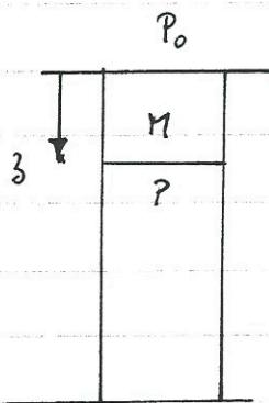
The mass  $M$  is supported by the pressure at depth  $z$ :
