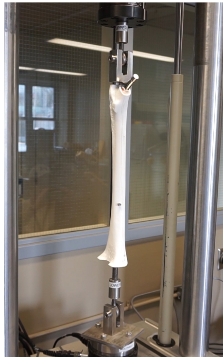
Figure 2. Pullout apparatus affixed to material testing system.
