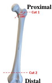
Fig. 2. Resections on synthetic femur (Sawbones, USA).
