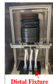
Fig. 3. Distal end fixture during constant compressive loading phase in incubator at 23°C.
