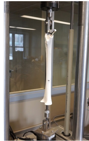
Figure 2. The assembled pullout apparatus affixed to a hydraulic test frame.
