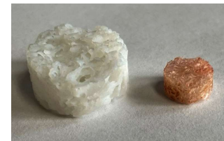
Figure 3: Real bone core (right) and corresponding 3D printed model (left).
