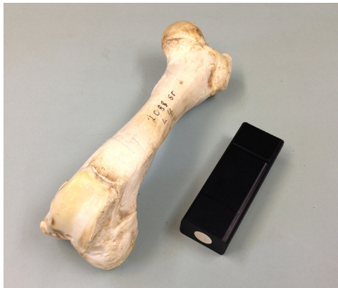
Fig. 3. Photo of a fabricated surrogate (Right) adjacent to an excised adult porcine femur (Left).
